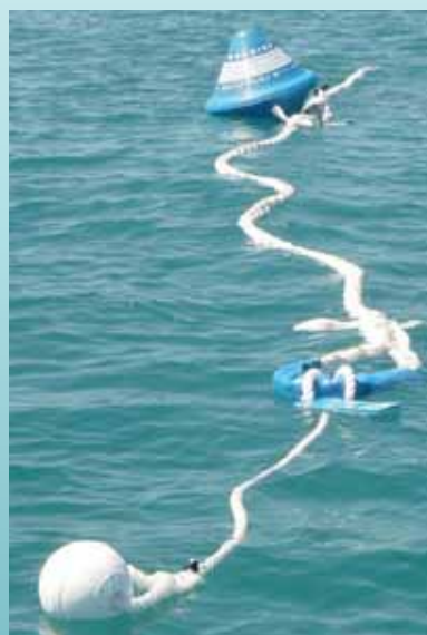
Moorings buoy, pick-up tag and pick-up line
